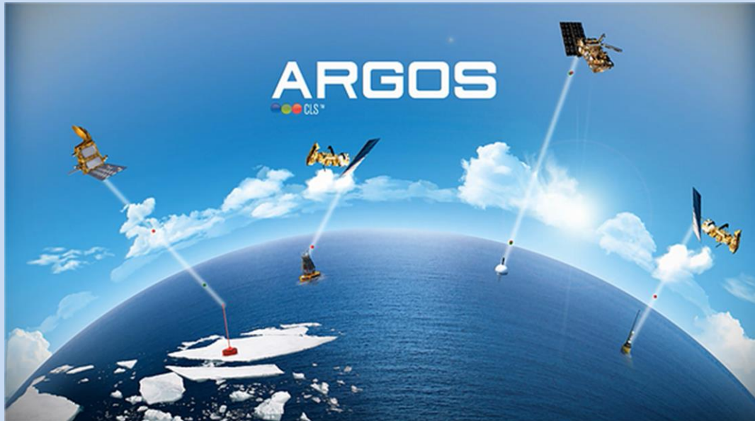
Figure 6: Collection of data from instrumentation by the ARGOS satellite system.
