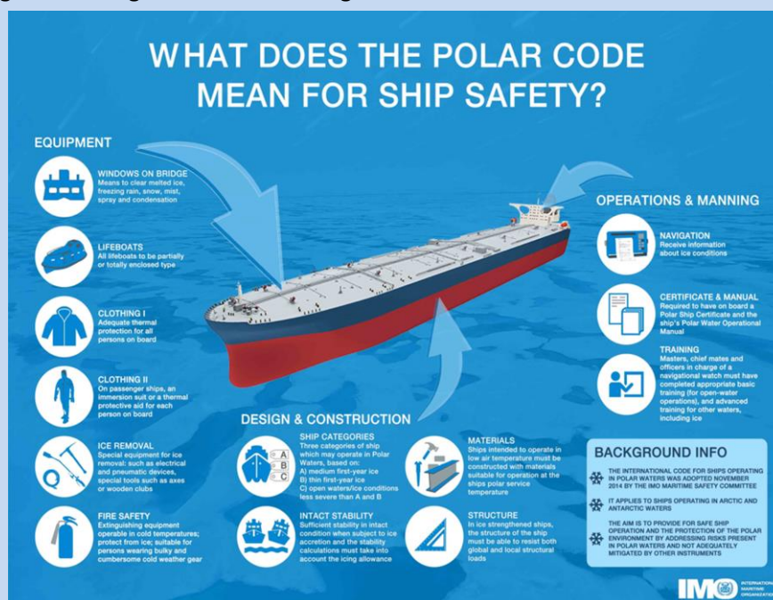
Figure 9: Summary graphic of IMO Polar Code requirements for ships operating in polar waters.
